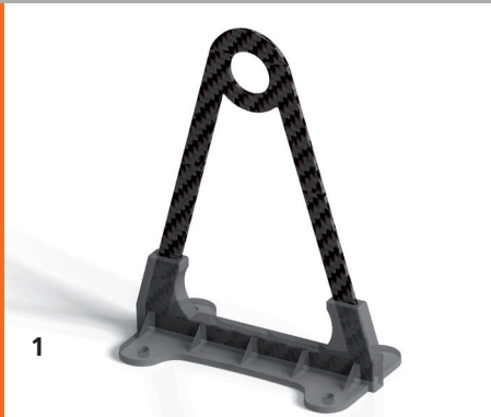
1 Specimen of a hybrid composite of aluminum and CFRP with a polymer based decoupling layer and produced in high-pressure die casting.
